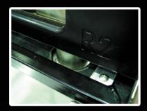
The R2 Aerial Incendiary Device incorporates a drip tray in the frame assembly, ensuring all fluids exit the aircraft via the Drop Tube. The unique Drop Tube Mounting Plate provides for ease of installation and removal.
