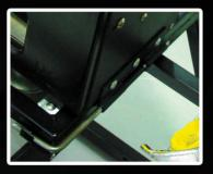
Pins holding the R2 Aerial Incendiary machine to the frame provide a secure and firm mounting, whilst allowing for quick removal of the device.
