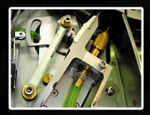
Glycol injection and Belt cutting are controlled mechanically, likewise, pumping is via by peristaltic action. This allows for very accurate dosing and reliability, ensuring the R2 Aerial Incendiary Device achieves a very high success rate every time.
